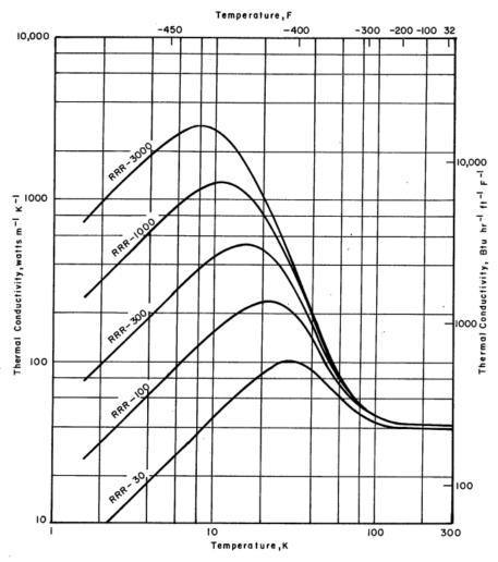
THERMAL CONDUCTIVITY VERSUS TEMPERATURE FOR COPPER
